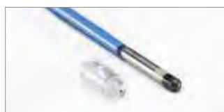
Semiflex Chamber (31010) Volume: 0.125 cm 3 Field size: (3 x 3) cm 2 ... (40 x 40) cm 2
